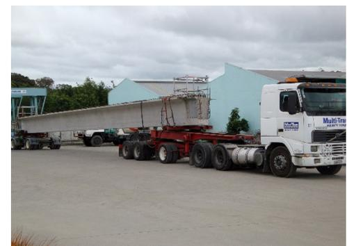
A completed concrete pre-stressed beam ready for transport.
